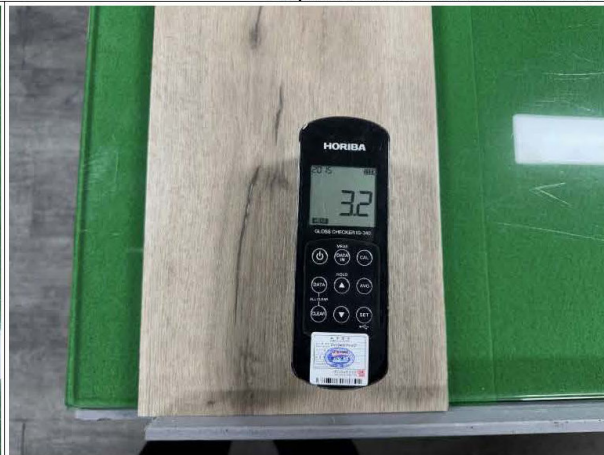
Check sheen level
