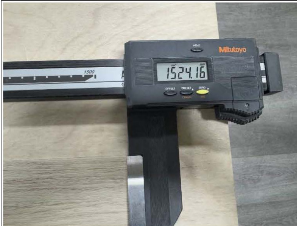
Check length of plank
