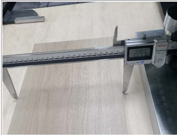
Shrinkage- Measure width after heating
