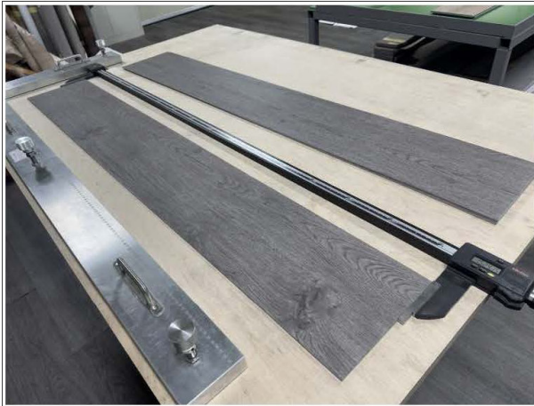
Check length of plank
