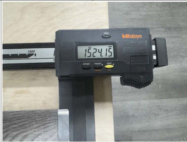
Check length of plank
