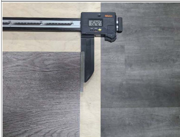
Shrinkage- Measure length before heating
