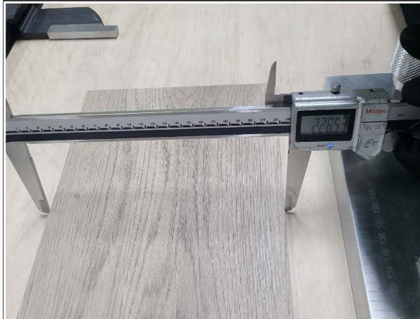
Shrinkage- Measure width after heating
