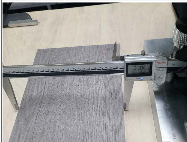
Shrinkage- Measure width after heating
