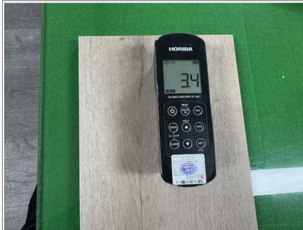
Check sheen level
