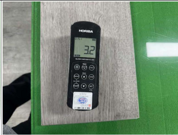
Check sheen level
