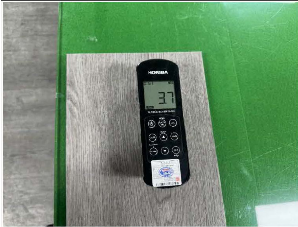
Check sheen level
