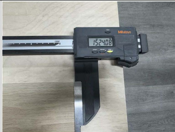
Check length of plank
