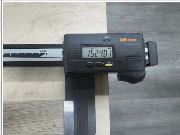
Check length of plank
