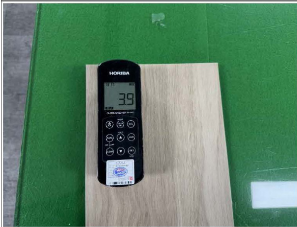
Check sheen level
