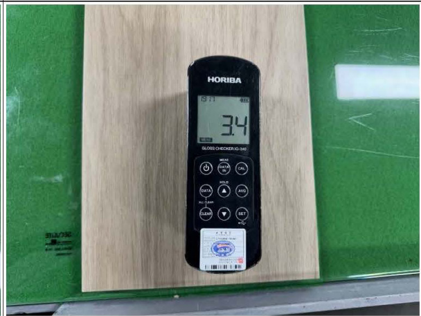
Check sheen level
